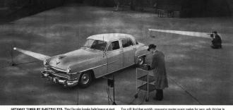
GETAWAY TIMED BY ELECTRIC EYE. This Chryster breaks light beams at start and finish of getaway test, while electronic machines measure time to a split second.
